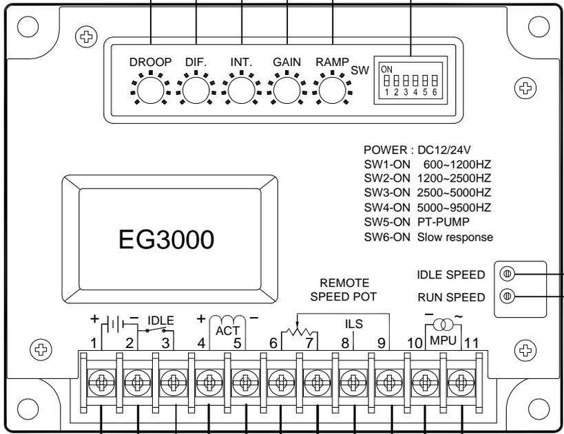
**IDLE SPEED : IDLE Speed Setting**
